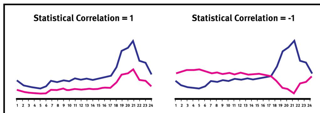
Evaluating similarity between two load profiles using statistical correlation between two data series
