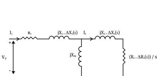
Electrical equivalent circuit for the induction motor taking into account parameters variation
