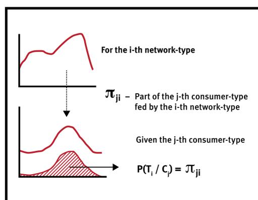
Definition of the " $\pi$ " variables, indicating how a customer-type will be fed by a network-type load profile
