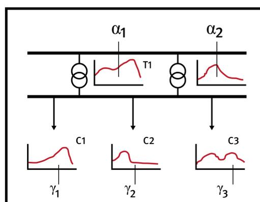
Two network-type load profiles and three customer-type load profiles
